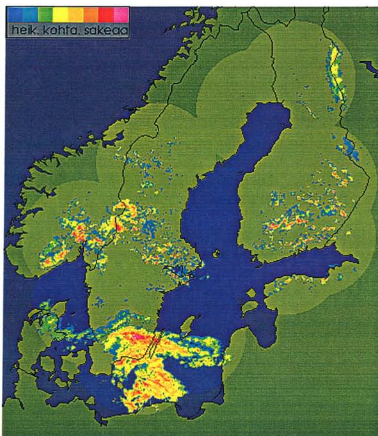
Figure 1.1 : NORDRAD reflectivity composite at 14 UTC on May 27, 1996. As it is a customer product, the scale explanation is in Finnish . The exact scale starts from -6 dBZ and one colour step is 6 dBZ.
